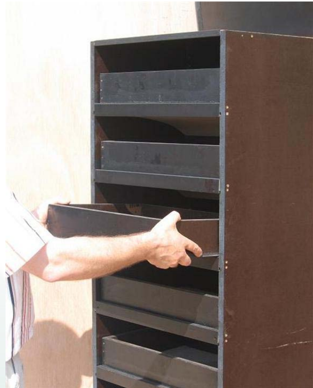
Air-inlet opens when tray is being placed
